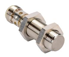
ProSense inductive proximity sensor, tubular, 12mm diameter x 45mm body, stainless steel housing, PNP, N.O. output, 4mm sensing distance, flush, 100 Hz switching frequency, IP65 IP66 IP67 IP68 IP69K, 4-pin M12 quick-disconnect.
