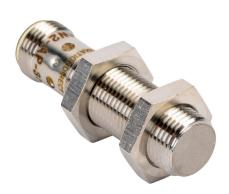
ProSense inductive proximity sensor, tubular, 12mm diameter x 45mm body, stainless steel housing, PNP, N.O. output, 4mm sensing distance, flush, 100 Hz switching frequency, IP65 IP66 IP67 IP68 IP69K, 4-pin M12 quick-disconnect.
