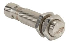
AutomationDirect inductive proximity sensor, tubular, 12mm diameter x 60mm body, stainless steel housing, PNP, N.O. output, 6mm sensing distance, flush, 400 Hz switching frequency, IP67, 4-pin M12 quick-disconnect.
