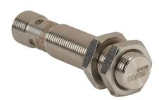
AutomationDirect inductive proximity sensor, tubular, 12mm diameter x 60mm body, stainless steel housing, NPN, N.O. output, 6mm sensing distance, flush, 400 Hz switching frequency, IP67, 4-pin M12 quick-disconnect.
