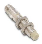
Micro Detectors inductive proximity sensor, tubular, 12mm diameter x 64.8mm body, stainless steel housing, PNP, N.O./N.C. complementary outputs, 4mm sensing distance, non-flush, 2 kHz switching frequency, IP67 IP68, 4-pin M12 quick-disconnect.
