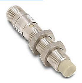
Micro Detectors inductive proximity sensor, tubular, 12mm diameter x 64.8mm body, stainless steel housing, PNP, N.O./N.C. complementary outputs, 4mm sensing distance, non-flush, 2 kHz switching frequency, IP67 IP68, 4-pin M12 quick-disconnect.
