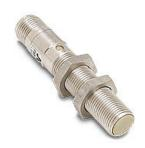
Micro Detectors inductive proximity sensor, tubular, 12mm diameter x 64.8mm body, stainless steel housing, PNP, N.O./N.C. complementary outputs, 2mm sensing distance, flush, 2 kHz switching frequency, IP67 IP68, 4-pin M12 quick-disconnect.
