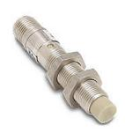
Micro Detectors inductive proximity sensor, tubular, 12mm diameter x 64.8mm body, stainless steel housing, NPN, N.O./N.C. complementary outputs, 4mm sensing distance, non-flush, 2 kHz switching frequency, IP67 IP68, 4-pin M12 quick-disconnect.
