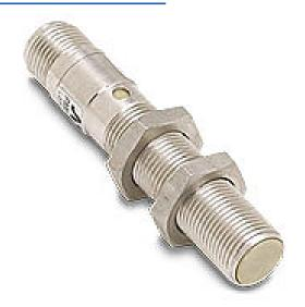
Micro Detectors inductive proximity sensor, tubular, 12mm diameter x 64.8mm body, stainless steel housing, NPN, N.O./N.C. complementary outputs, 2mm sensing distance, flush, 2 kHz switching frequency, IP67 IP68, 4-pin M12 quick-disconnect.
