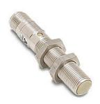
Micro Detectors inductive proximity sensor, tubular, 12mm diameter x 64.8mm body, stainless steel housing, NPN, N.O./N.C. complementary outputs, 2mm sensing distance, flush, 2 kHz switching frequency, IP67 IP68, 4-pin M12 quick-disconnect.
