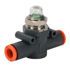
NITRA pneumatic push-to-connect fitting, inline pressure indicator, technopolymer body, (1) 5/16in (8mm) push-to-connect inlet(s), (1) 5/16in (8mm) push-to-connect outlet(s), 29-145 psi range, green indication.
