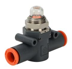
NITRA pneumatic push-to-connect fitting, inline pressure indicator, technopolymer body, 5/16in (8mm) tube inlet(s), 5/16in (8mm) tube outlet(s), 29-145 psi range, orange indication.
