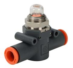
NITRA pneumatic push-to-connect fitting, inline pressure indicator, technopolymer body, (1) 5/16in (8mm) push-to-connect inlet(s), (1) 5/16in (8mm) push-to-connect outlet(s), 29-145 psi range, orange indication.
