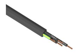
Southwire flexible power/control cable, unshielded, 4 conductors (includes ground), 8 AWG, bare copper, PVC/Nylon conductor insulation material, black with white numbers and green/yellow ground, TPE jacket, black, cut to length.
