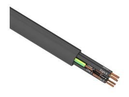
Southwire flexible power/control cable, unshielded, 9 conductors (includes ground), 18 AWG, bare copper, PVC/Nylon conductor insulation material, black with white numbers and green/yellow ground, TPE jacket, black, cut to length.
