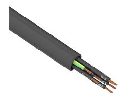
Southwire flexible power/control cable, unshielded, 7 conductors (includes ground), 18 AWG, bare copper, PVC/Nylon conductor insulation material, black with white numbers and green/yellow ground, TPE jacket, black, cut to length.
