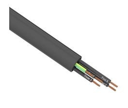
Southwire flexible power/control cable, unshielded, 5 conductors (includes ground), 18 AWG, bare copper, PVC/Nylon conductor insulation material, black with white numbers and green/yellow ground, TPE jacket, black, cut to length.
