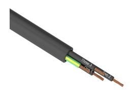
Southwire flexible power/control cable, unshielded, 4 conductors (includes ground), 18 AWG, bare copper, PVC/Nylon conductor insulation material, black with white numbers and green/yellow ground, TPE jacket, black, cut to length.
