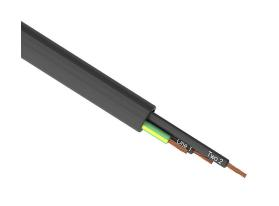
Southwire flexible power/control cable, unshielded, 3 conductors (includes ground), 18 AWG, bare copper, PVC/Nylon conductor insulation material, black with white numbers and green/yellow ground, TPE jacket, black, cut to length.
