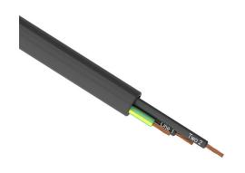
Southwire flexible power/control cable, unshielded, 3 conductors (includes ground), 18 AWG, bare copper, PVC/Nylon conductor insulation material, black with white numbers and green/yellow ground, TPE jacket, black, cut to length.
