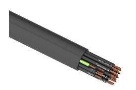
Southwire flexible power/control cable, unshielded, 25 conductors (includes ground), 18 AWG, bare copper, PVC/ Nylon conductor insulation material, black with white numbers and green/yellow ground, TPE jacket, black, cut to length.
