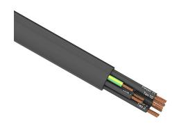
Southwire flexible power/control cable, unshielded, 12 conductors (includes ground), 18 AWG, bare copper, PVC/ Nylon conductor insulation material, black with white numbers and green/yellow ground, TPE jacket, black, cut to length.
