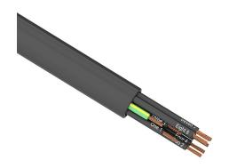
Southwire flexible power/control cable, unshielded, 9 conductors (includes ground), 16 AWG, bare copper, PVC/Nylon conductor insulation material, black with white numbers and green/yellow ground, TPE jacket, black, cut to length.
