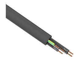
Southwire flexible power/control cable, unshielded, 5 conductors (includes ground), 16 AWG, bare copper, PVC/Nylon conductor insulation material, black with white numbers and green/yellow ground, TPE jacket, black, cut to length.
