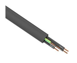
Southwire flexible power/control cable, unshielded, 5 conductors (includes ground), 16 AWG, bare copper, PVC/Nylon conductor insulation material, black with white numbers and green/yellow ground, TPE jacket, black, cut to length.
