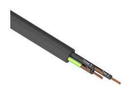
Southwire flexible power/control cable, unshielded, 4 conductors (includes ground), 16 AWG, bare copper, PVC/Nylon conductor insulation material, black with white numbers and green/yellow ground, TPE jacket, black, cut to length.
