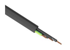
Southwire flexible power/control cable, unshielded, 3 conductors (includes ground), 16 AWG, bare copper, PVC/Nylon conductor insulation material, black with white numbers and green/yellow ground, TPE jacket, black, cut to length.
