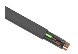
Southwire flexible power/control cable, unshielded, 12 conductors (includes ground), 16 AWG, bare copper, PVC/ Nylon conductor insulation material, black with white numbers and green/yellow ground, TPE jacket, black, cut to length.
