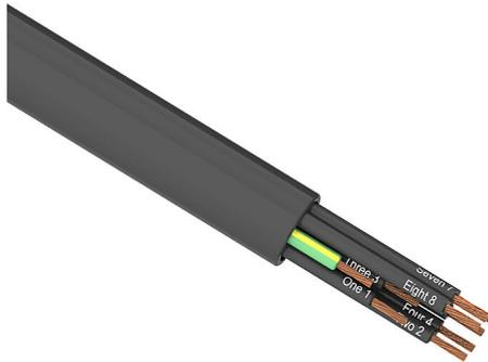
Southwire flexible power/control cable, unshielded, 9 conductors (includes ground), 14 AWG, bare copper, PVC/Nylon conductor insulation material, black with white numbers and green/yellow ground, TPE jacket, black, cut to length.
