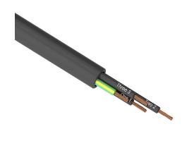
Southwire flexible power/control cable, unshielded, 4 conductors (includes ground), 14 AWG, bare copper, PVC/Nylon conductor insulation material, black with white numbers and green/yellow ground, TPE jacket, black, cut to length.
