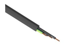
Southwire flexible power/control cable, unshielded, 3 conductors (includes ground), 14 AWG, bare copper, PVC/Nylon conductor insulation material, black with white numbers and green/yellow ground, TPE jacket, black, cut to length.
