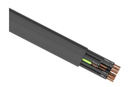
Southwire flexible power/control cable, unshielded, 18 conductors (includes ground), 14 AWG, bare copper, PVC/ Nylon conductor insulation material, black with white numbers and green/yellow ground, TPE jacket, black, cut to length.
