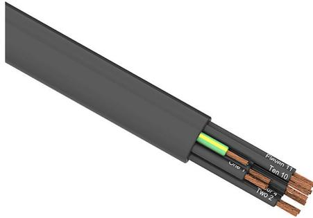
Southwire flexible power/control cable, unshielded, 12 conductors (includes ground), 14 AWG, bare copper, PVC/Nylon conductor insulation material, black with white numbers and green/yellow ground, TPE jacket, black, cut to length.
