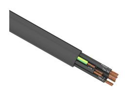
Southwire flexible power/control cable, unshielded, 12 conductors (includes ground), 14 AWG, bare copper, PVC/ Nylon conductor insulation material, black with white numbers and green/yellow ground, TPE jacket, black, cut to length.
