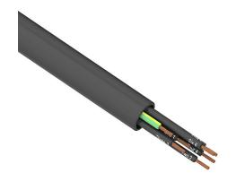
Southwire flexible power/control cable, unshielded, 7 conductors (includes ground), 12 AWG, bare copper, PVC/Nylon conductor insulation material, black with white numbers and green/yellow ground, TPE jacket, black, cut to length.
