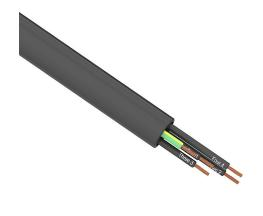
Southwire flexible power/control cable, unshielded, 5 conductors (includes ground), 12 AWG, bare copper, PVC/Nylon conductor insulation material, black with white numbers and green/yellow ground, TPE jacket, black, cut to length.
