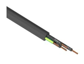
Southwire flexible power/control cable, unshielded, 4 conductors (includes ground), 12 AWG, bare copper, PVC/Nylon conductor insulation material, black with white numbers and green/yellow ground, TPE jacket, black, cut to length.
