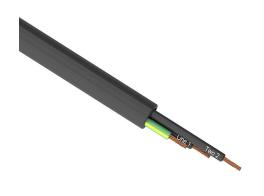
Southwire flexible power/control cable, unshielded, 3 conductors (includes ground), 12 AWG, bare copper, PVC/Nylon conductor insulation material, black with white numbers and green/yellow ground, TPE jacket, black, cut to length.
