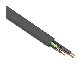
Southwire flexible power/control cable, unshielded, 5 conductors (includes ground), 10 AWG, bare copper, PVC/Nylon conductor insulation material, black with white numbers and green/yellow ground, TPE jacket, black, cut to length.
