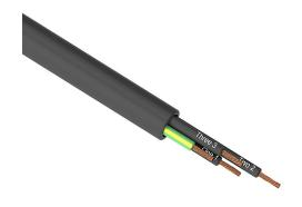
Southwire flexible power/control cable, unshielded, 4 conductors (includes ground), 10 AWG, bare copper, PVC/Nylon conductor insulation material, black with white numbers and green/yellow ground, TPE jacket, black, cut to length.
