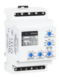
ProSense phase monitor relay, 3-phase, 35mm DIN rail mount, 460-600 VAC input voltage, DPDT, 10A contact rating, screw terminal(s), LED indicator(s), phase reversal, phase loss, phase unbalance, overvoltage and undervoltage protection.
