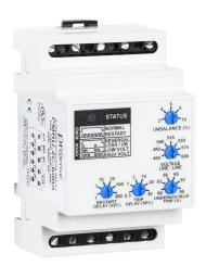
ProSense phase monitor relay, 3-phase, 35mm DIN rail mount, finger-safe, 460-600 VAC input voltage, DPDT, 10A contact rating, screw terminal(s), LED indicator(s), phase reversal, phase loss, phase unbalance, overvoltage and undervoltage protection.
