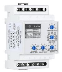
ProSense phase monitor relay, 3-phase, 35mm DIN rail mount, 190-500 VAC input voltage, DPDT, 10A contact rating, screw terminal(s), LED indicator(s), phase reversal, phase loss, phase unbalance, overvoltage and undervoltage protection.
