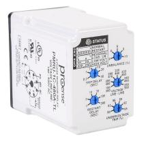
ProSense phase monitor relay, 3-phase, socket mount, 190-500 VAC input voltage, SPDT, 10A contact rating, 8-pin, LED indicator(s), phase reversal, phase loss, phase unbalance, overvoltage and undervoltage protection.
