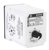
ProSense phase monitor relay, 3-phase, socket mount, 240 VAC input voltage, SPDT, 10A contact rating, 8-pin, LED indicator(s), phase reversal, phase loss and undervoltage protection.
