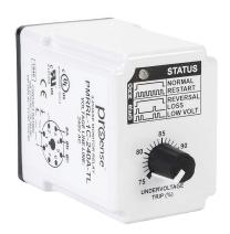
ProSense phase monitor relay, 3-phase, socket mount, finger-safe, 240 VAC input voltage, SPDT, 10A contact rating, 8-pin, LED indicator(s), phase reversal, phase loss and undervoltage protection.
