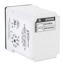
ProSense phase monitor relay, 3-phase, socket mount, fingersafe, 190-500 VAC input voltage, SPDT, 10A contact rating, 8-pin, LED indicator(s), phase reversal protection.
