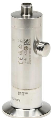
Endress+Hauser Cerabar pressure transmitter, 0 to 15 psig range, +/- 0.3% accuracy, stainless steel sensing element, Output: 4-20 mA, Output 2: IO-Link, 1-1/2in sanitary tri-clamp process connection, 18-30 VDC operating voltage, 4-pin M12 quick-disconnect.
