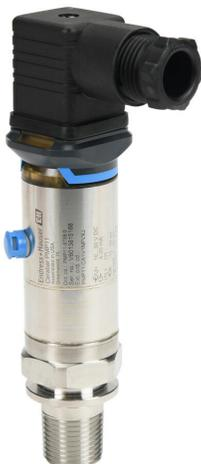
Endress+Hauser Cerabar pressure transmitter, 0 to 90 psig range, +/- 0.5% accuracy, stainless steel sensing element, 4-20 mA analog output, 1/2in male NPT or 1/4in female NPT process connection, 10-30 VDC operating voltage, ISO4400 valve plug.
