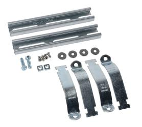
Integra pole mounting kit, accommodates 4in pole diameter, galvanized steel components and zinc-plated steel fasteners. For use with 10in wide Premium series polycarbonate enclosures.
