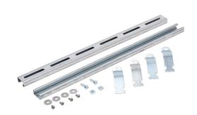
Integra pole mounting kit, accommodates 3in pole diameter, galvanized steel components and zinc-plated steel fasteners. For use with 24in wide Genesis series polycarbonate enclosures.
