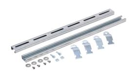
Integra pole mounting kit, accommodates 2in pole diameter, galvanized steel components and zinc-plated steel fasteners. For use with 24in wide Genesis series polycarbonate enclosures.
