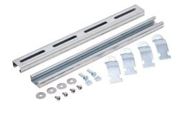
Integra pole mounting kit, accommodates 2in pole diameter, galvanized steel components and zinc-plated steel fasteners. For use with 16in wide Premium series polycarbonate enclosures.
