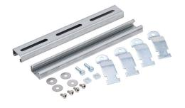
Integra pole mounting kit, accommodates 2in pole diameter, galvanized steel components and zinc-plated steel fasteners. For use with 12in wide Premium series polycarbonate enclosures.
