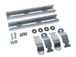
Integra pole mounting kit, accommodates 2in pole diameter, galvanized steel components and zinc-plated steel fasteners. For use with 10in wide Premium series polycarbonate enclosures.
