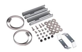
Integra pole mounting kit, accommodates 9-1/2 to 12in pole diameter, galvanized steel components and zinc-plated steel fasteners. For use with 6in wide Impact series polycarbonate enclosures.
