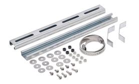
Integra pole mounting kit, accommodates 9-1/2 to 12in pole diameter, galvanized steel components and zinc-plated steel fasteners. For use with 16in wide Genesis series polycarbonate enclosures.
