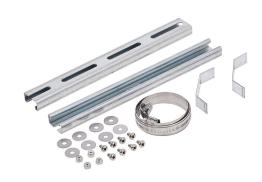
Integra pole mounting kit, accommodates 9-1/2 to 12in pole diameter, galvanized steel components and zinc-plated steel fasteners. For use with 14in wide Premium series polycarbonate enclosures.
