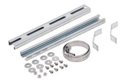
Integra pole mounting kit, accommodates 9-1/2 to 12in pole diameter, galvanized steel components and zinc-plated steel fasteners. For use with 14in wide Premium series polycarbonate enclosures.
