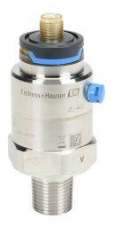
Endress+Hauser Cerabar pressure transmitter, 0 to 150 psig range, +/- 0.3% accuracy, ceramic sensing element, FKM seal(s), 4-20 mA analog output, 1/2in male NPT or 1/4in female NPT process connection, 10-30 VDC operating voltage, 4-pin M12 quick-disconnect.
